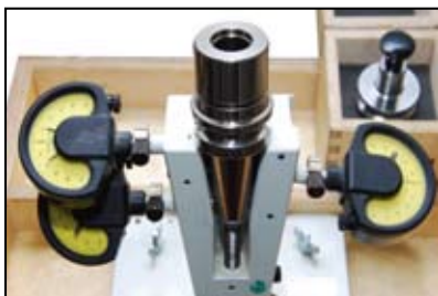
7: 24锥检具图(德国Diebold刀柄检具) Picture of 7:24 taper inspection tool (German Diebold collet chuck inspection tool)
